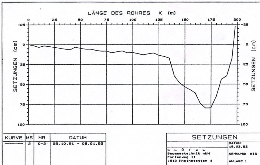
Settlement course after comparison of measuring series between first sequence measurement and zero measurement
