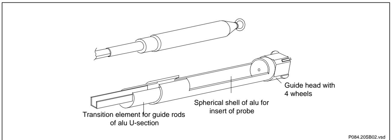
Connection piece probe - rods
