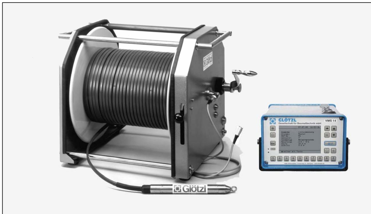
The hydrostatic profile gauge has been designed for measurement of the absolute height in horizontal resp. slightly horizontally inclined tubes. When passing the tubes with the measuring probe, the height difference between probe and a reference benchmark at tube beginning is determined at selected points. By comparison of two measuring series at different times, you get the settlement of the tube.
