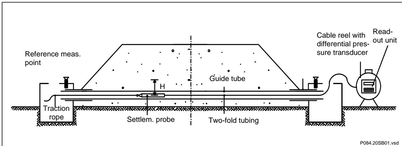
Installation example with double-sided access of measuring tube, measurement execution with traction rope
