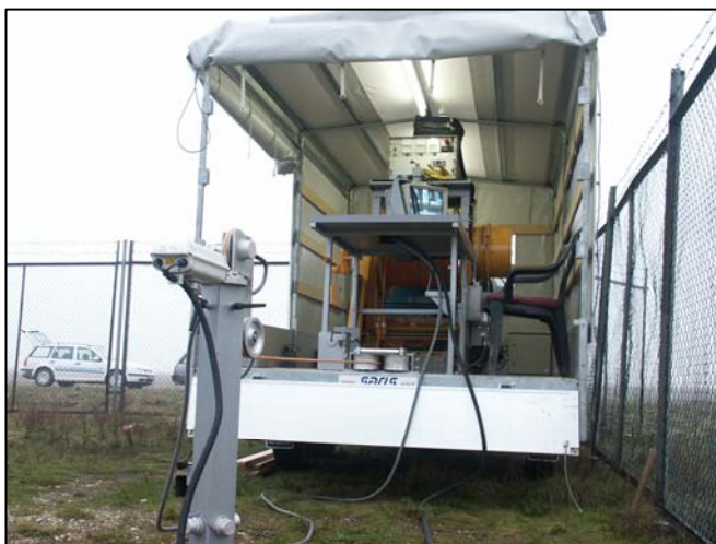
Measuring device during measurement of a 564 m deep level
