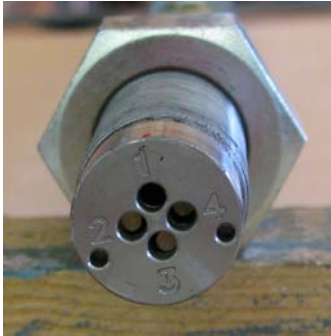
Figure 1: Standard measuring head MA25 for measurement with a dial gauge
