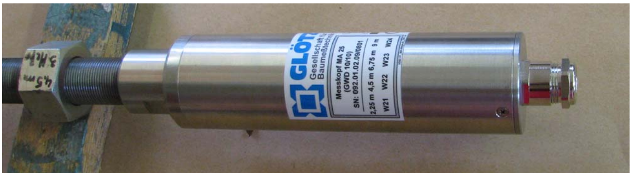
Figure 3: Measuring head with distant reading, completely mounted
