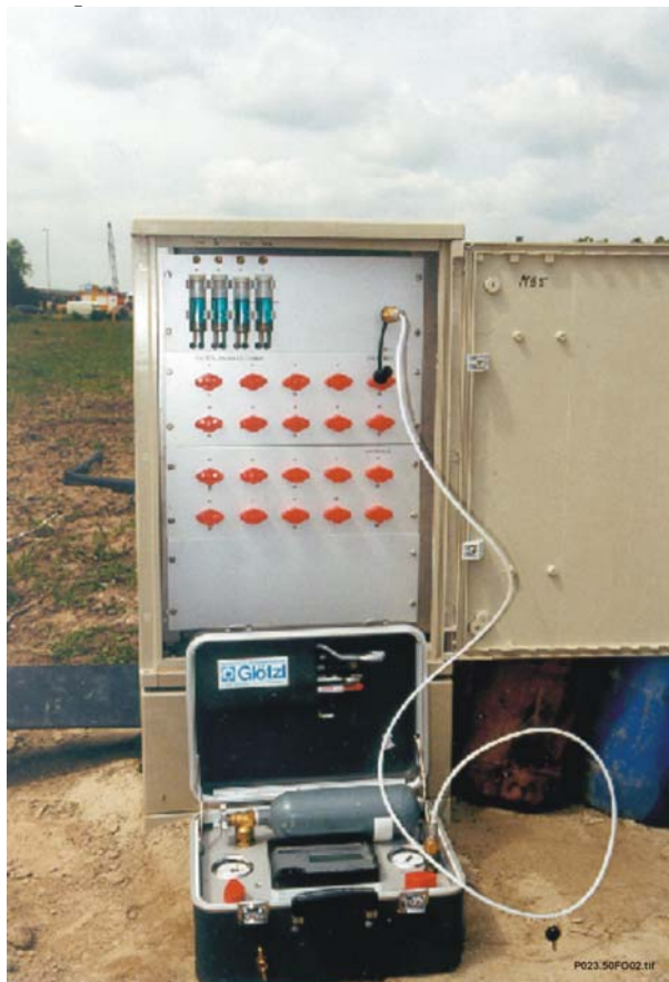
Figure: Measuring station with pneumatic measuring device ALR
