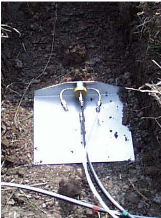
Figure: Settlement cell type TA 4 30/30 LF 20 with settlement plate
