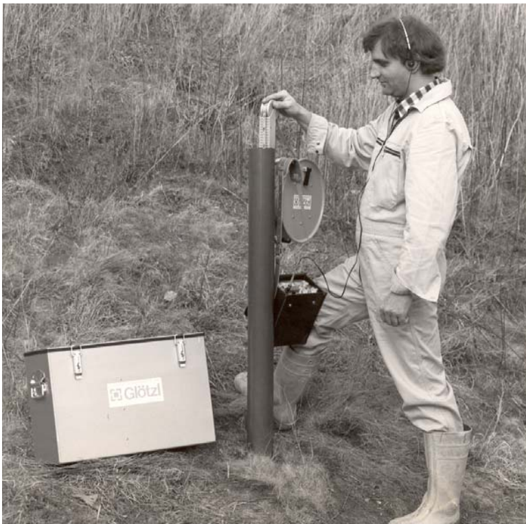
Figure.: Measurement with metal plate settlement indicator
