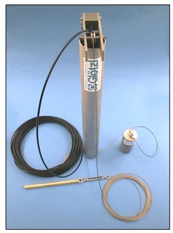
A stainless steel wire is prestressed between two fixed points (e.g. cemented bolts) by means of a tension weight. The changes in length and distance between the fixed points are recorded by a distance measurement at the tension weight.
