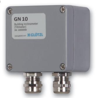
The GN 10 compact building inclinometer features precise inclinometer sensors with a restricted measuring range of  $\pm 10^{\circ}$  and a resolution of 0.02 mm/m for measured values. It is used to record inclination changes in buildings. Equipped with a sensor for measuring axis x and a temperature sensor, the GN 10/1 tiltmeter records inclinations at right angles to the mounting surface, while the GN 10/2 2-axis sensor measures in both x and y directions.
