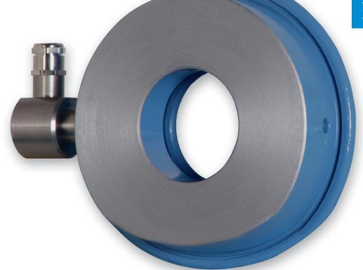
The compact GLÖTZL anchor load cell with integrated distribution plate and electronic transducer comprises a defined area sensor pad made up of two flexurally stiff discs that are moveable through annular grooves around their circumference. The pressure chamber is filled with hydraulic fluid that is connected to a pressure sensor.
